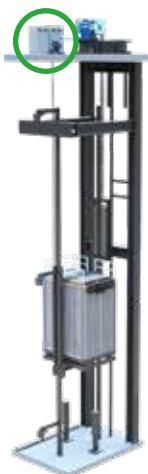
Machine Room Drive on the Rooftop
