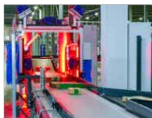
DWS front-end belt conveyor
